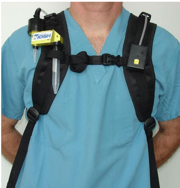
NIOSH sampler worn by a healthcare worker. The sampling pump is in the backpack behind the worker. The black box on the left shoulder turns the pump on and off. The yellow button pauses the pump for 60 seconds and then automatically starts it again. This feature is used by healthcare workers when they need a very quiet environment such as when using a stethoscope.
