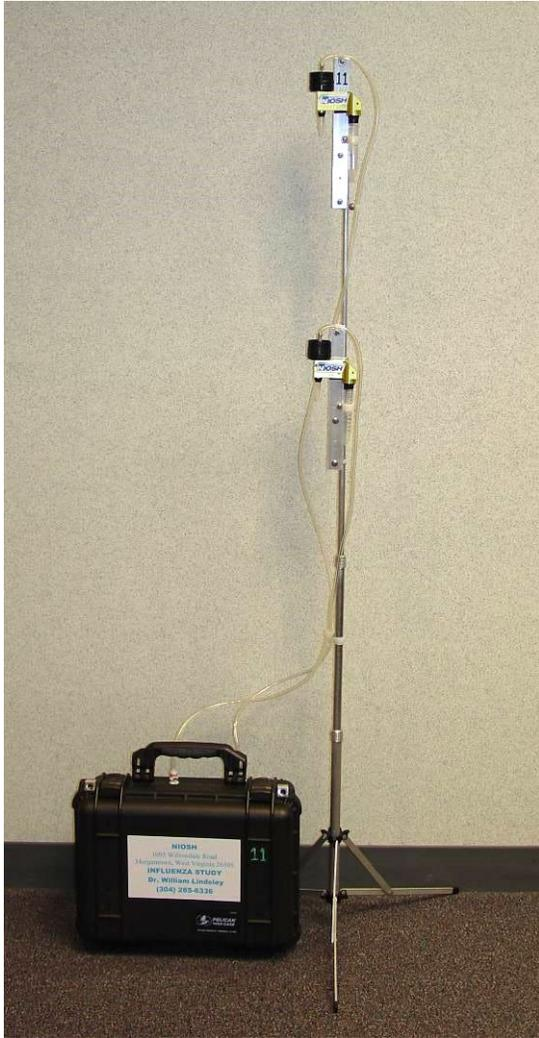
Two NIOSH samplers are shown on a tripod in a healthcare facility. The black case on the floor contains two sampling pumps that pull air through the samplers.
